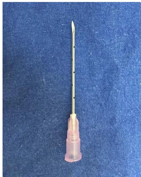
**FIGURE 2.** The perforated needle used in our intramedullary venous drainage system. The holes are 0.2 mm in diameter and are opened with a wire erosion machine.
